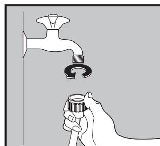
The water inlet valve of the washing machine must be connected to a cold-water supply.
